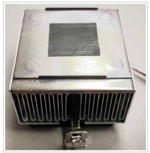
Well designed: Elan Vital's cooler is equipped with a copper heat spreader. In addition to that, it has cooling foils made of aluminum.
