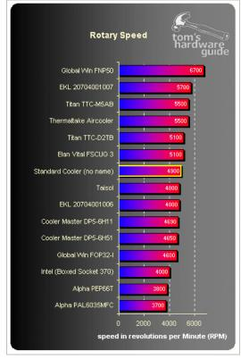
The "small" Global Win is the fastest cooler with 6700 rpm. The others lie between 4000 and 5000 rpms.
