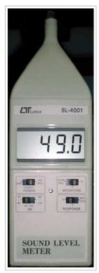
With this measuring device we determined the noise level (dBA) of all coolers.
