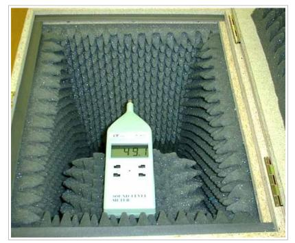
Our miniature sound chamber has enough space for a motherboard, hard disk or even a CPU cooler. The noise level is determined in the middle above the CPU cooler at a constant distance.
